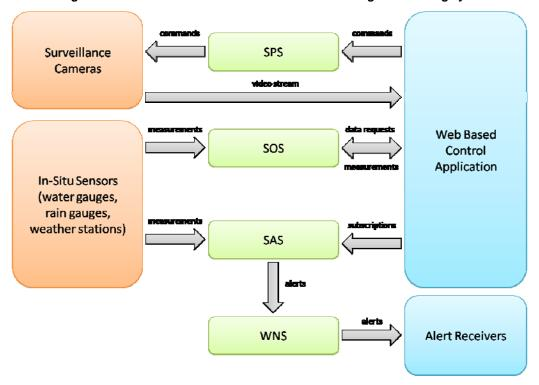
Figure 7: Architecture overview of the flood monitoring and warning system
